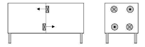
Figure A.1 — Arrangement with 4 fans, principle
