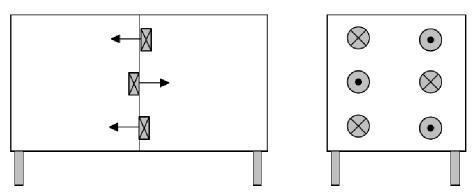
Figure A.2 — Arrangement with 6 fans, principle
